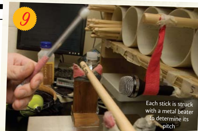
Pitch- and weight-matched sticks are paired and sleeved
